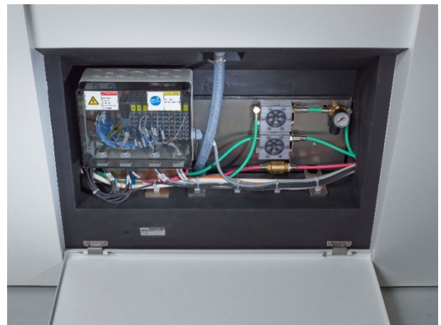
Figure 1: Smartbox implemented in the machine base
