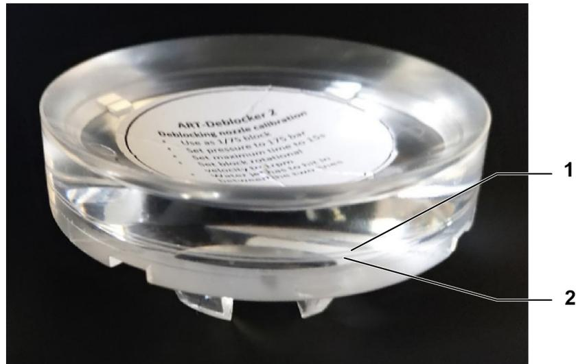
On this calibration block there are two marked lines (see Fig. 3-64, Item 1 and 2) between which the water jet should shoot during the deblocking process. These two calibration lines can be used to determine the water jet offset.
