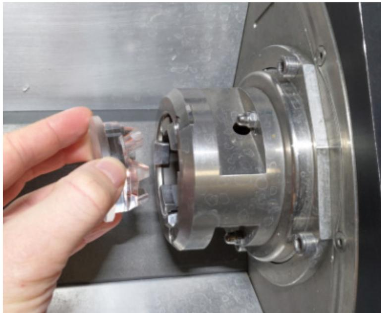
Fig. 3-70 Calibration block 1 in chamber 1
