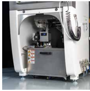
Compact footprint with polish tank conveniently fits inside the machine
