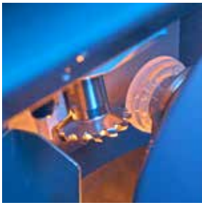
Fast milling process with 24,000 RPM.
