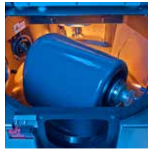
Orbital alignment of tool axes with robust work-piece spindle (B-axis).
