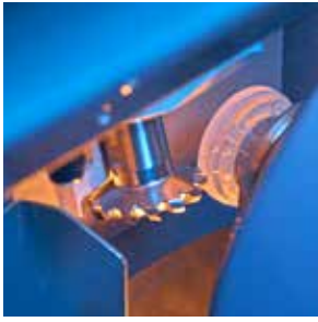
Fast milling process with 35,000 RPM, cribbing, chamfering and milling in less than 10 seconds.
