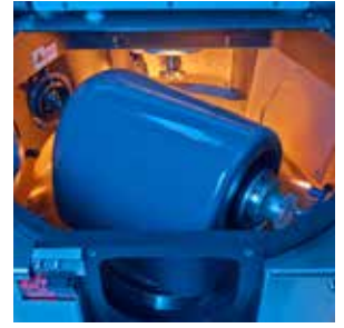
Orbital alignment of tool axes with robust work-piece spindle (B-axis).
