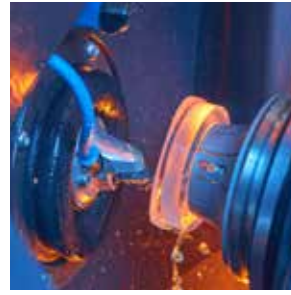
Through Tool Cooling cools down cutting point of the tool.
