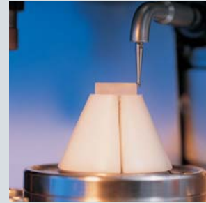
Measuring the lens diameter and the centre thickness with the integrated measuring system
