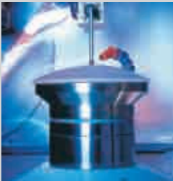
Integrated measuring system for centre thickness & lens diameter
