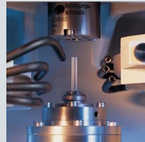
Special applications – alternatively use collet chucks to process special lenses
