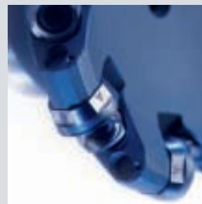
Effective: The cutting tips can be rotated 7 times and re-trued 3 to 4 times
