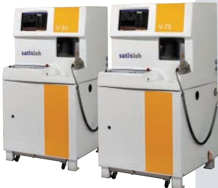
Flexible: The V-50 / V-75 process plastic and aluminium lap and polishing tools
