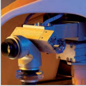
Fast lens loading system
