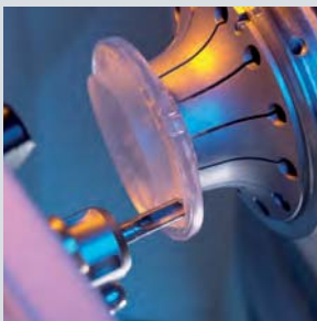
Cribbing and beveling of small lens diameters using PCD milling cutter
