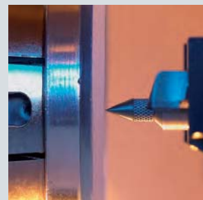
Engraving tool for semi visible markings
