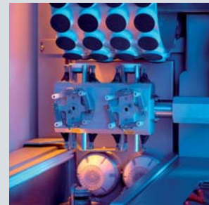
Polishing tool drum holds 72 polishing tools of 7 different curvatures
