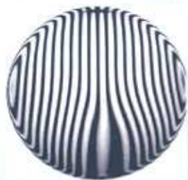
Distorted image of projected fringe image on surface to be measured
