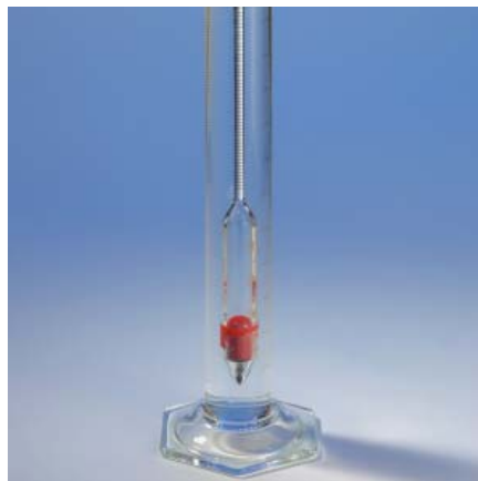
Measuring spindle with matching measuring cylinder (250 ml) to ascertain the concentration of polishing slurries.
