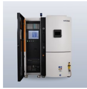
Control rack detachable from vacuum chamber frame for easy placement
